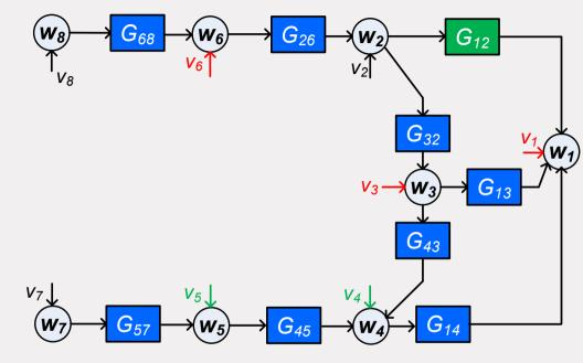
Network with  $v_1$  correlated with  $v_3$  and  $v_6$ .  $v_4$  correlated with  $v_5$ .
